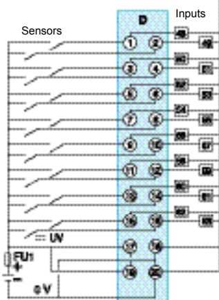
FU1: 0.5 A fast-blow fuse
